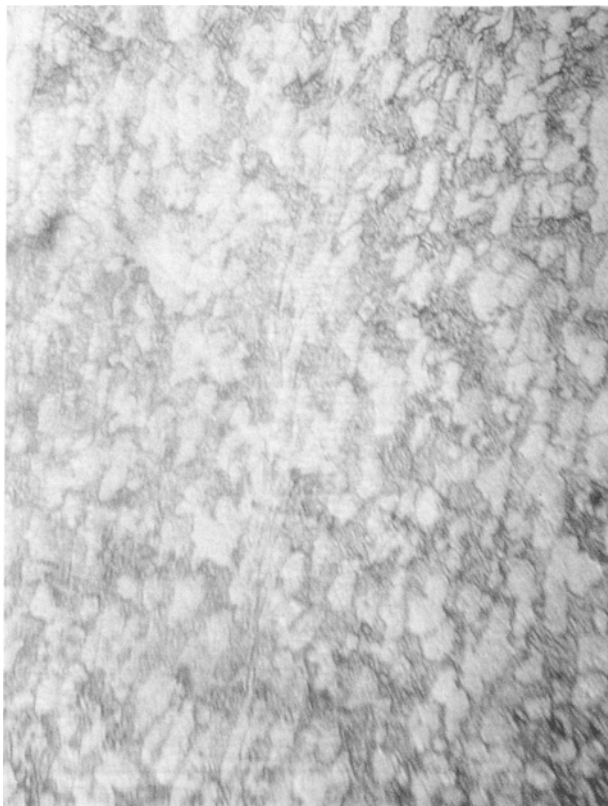
Fig. 11 Deformed band formed in titanium. 200x
